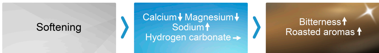
Figure 12: Softening reduces the calcium ( \text{Ca}^{2+} ) and magnesium ions ( \text{Mg}^{2+} ) in the water and increases the sodium ions ( \text{Na}^+ ) without affecting the amount of hydrogen carbonate ( \text{HCO}_3^- ) present.
