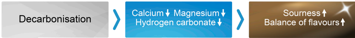
Figure 8: Decarbonisation reduces the amounts of calcium ( Ca^{2+} ), magnesium ( Mg^{2+} ) and ultimately also hydrogen carbonate ( HCO_3^- ) present in the water. This can result in increased perception of the acids and improve the flavour balance of the coffee.
