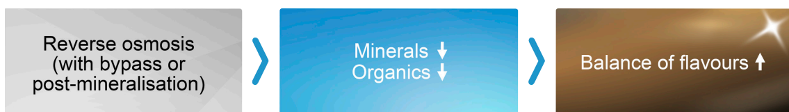
Figure 14: Reverse osmosis eliminates almost all minerals and organics from the water. This reduces the extent to which these substances detract from a balanced coffee flavour.
