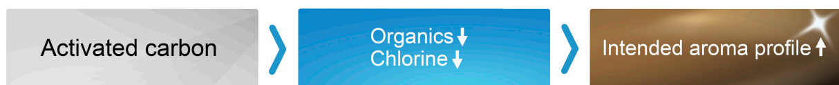
Figure 4: Activated carbon can reduce substances in the water that could otherwise detract from the desired and expected aroma profile of the coffee.
